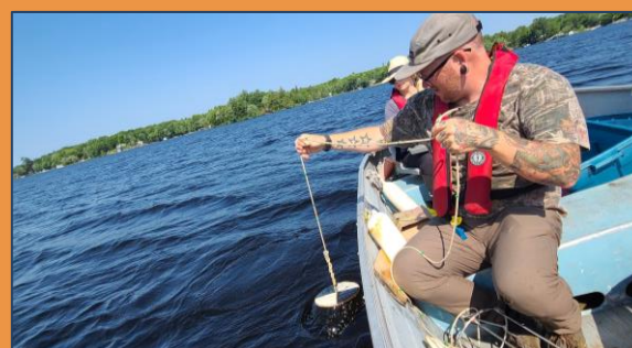
Measuring clarity with a Secchi disk
