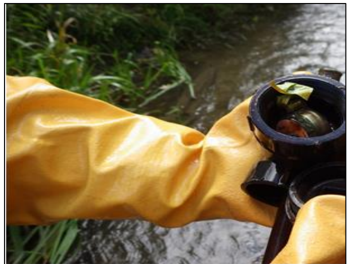
Temperature logger housing unit retrieval for data download
