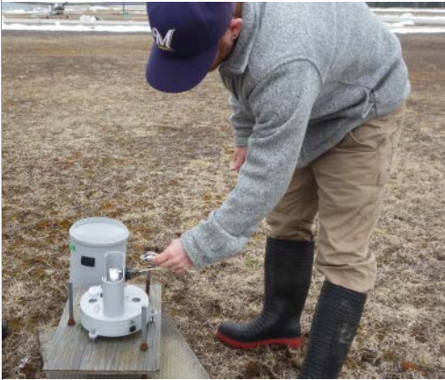
Fleming College Coop Student installing a rain gauge at Huronia Airport
