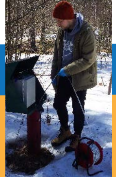
Monitoring Well Level Measurement
