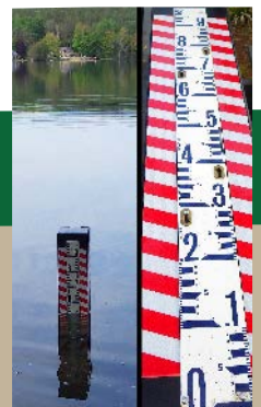
Farlain Lake Water Level Gauge
