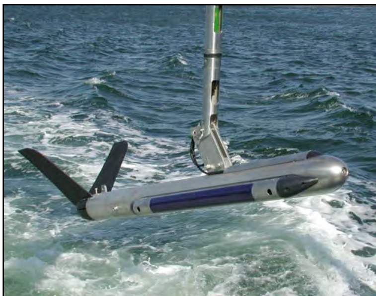
Figure 2. Image of L3-Klein System 3000 Towfish (courtesy Klein Marine, Inc.) Towfish resting in transport cradle ready for deployment during the Severn Sound study (photo Severn Sound Survey 2015)
