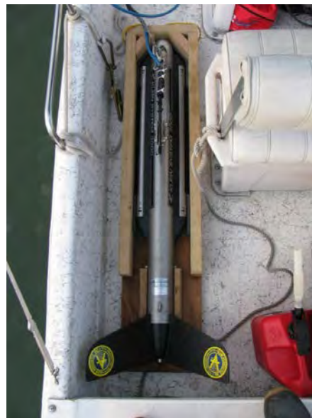
Figure 2. Image of L3-Klein System 3000 Towfish (courtesy Klein Marine, Inc.) Towfish resting in transport cradle ready for deployment during the Severn Sound study (photo Severn Sound Survey 2015)
