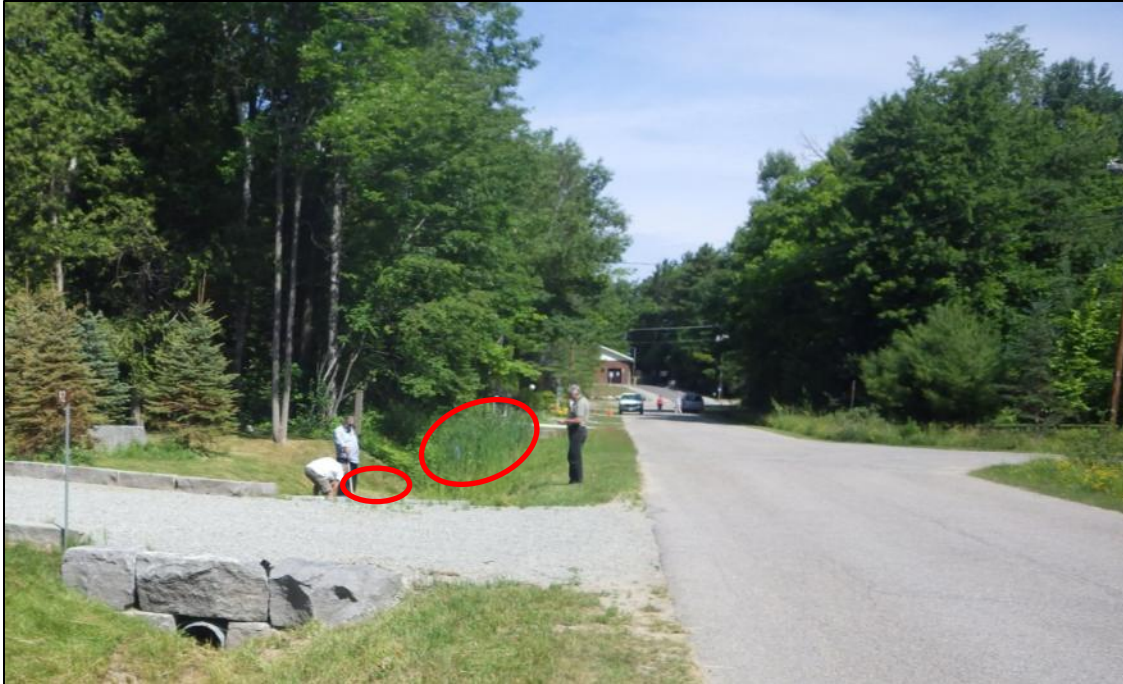
Jul 6 upstream of DB5 - Sump pump discharge on left, wet spot at right; both contributing to flow at DB5 during this dry period.
