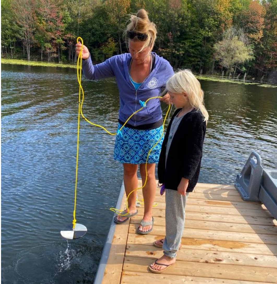
Shore Watch volunteers Alli and Abby Kornlyo measuring water clarity with a Secchi disk.
