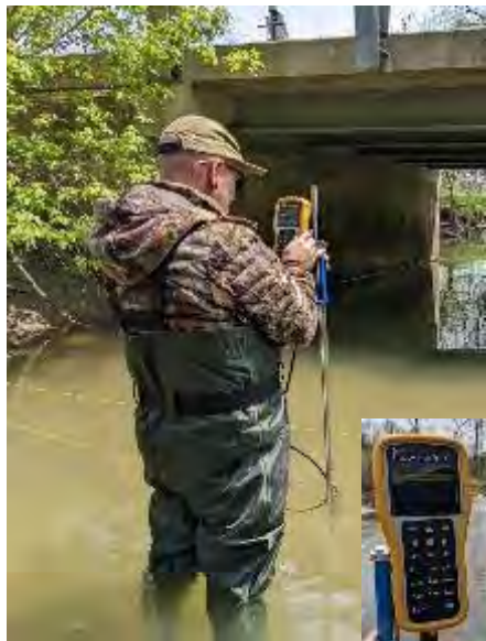
Recording flow with new flowmeter
