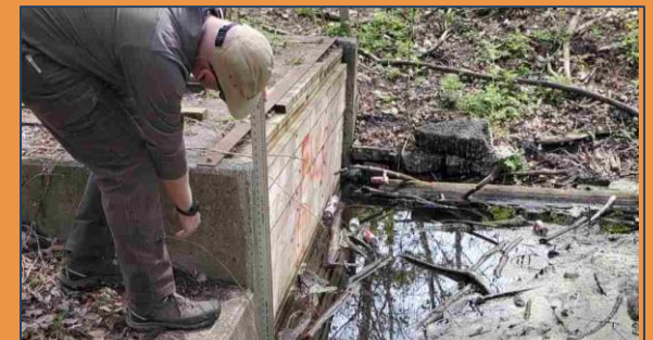
Staff measuring outlet water levels
