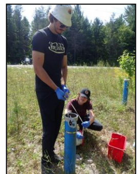
Collecting manual groundwater level readings
