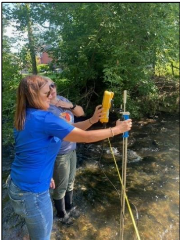
SSEA Board member Springwater Twp Councillor Alexander using a flow meter at the Stormwater Monitoring demonstration.
