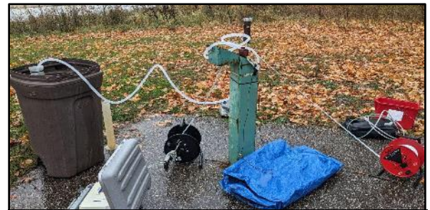
Purging Sundowner well in the Town of Midland, before collecting a chemistry sample
